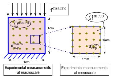
$\Omega^{\text{macro}}: 0.01 \times 0.01 \ m^2$  meshed with a 10×10-points grid yielding a spatial resolution of  $10^{-3} \times 10^{-3} \ m^2$ .
