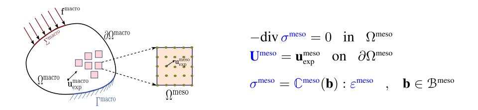
• Macroscopic-mesoscopic numerical indicator,  $\mathcal{J}_3(\mathbf{a}, \mathbf{b})$ , minimizes the distance between the macro elasticity tensor  $\mathbb{C}^{\text{macro}}(\mathbf{a})$  at macroscale and the effective elasticity tensor  $\mathbb{C}^{\text{eff}}(\mathbf{b})$  constructed by a stochastic homogenization using the RVE  $\Omega^{\text{meso}}$ :
