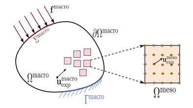
The stochastic homogenization (from meso to macro) is formulated in homogeneous constraints (that is better adapted for the 2D plane stresses) with  $\sigma^{\text{meso}} = \mathbb{C}^{\text{meso}}(\mathbf{b}) : \varepsilon^{\text{meso}}$ .
