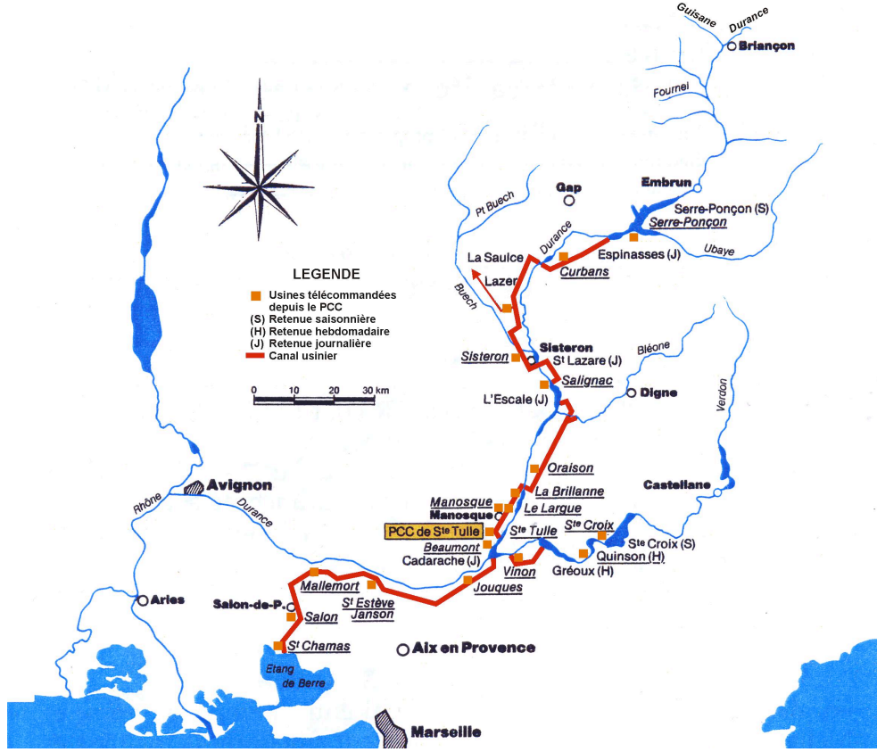
Figure 1.5: Chains of dams in France
