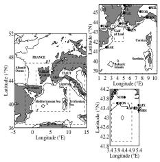
The MM5 model is run for 3 days between March 23rd and 25th, 1998 over the 3 nested domains with 3 with respective horizontal resolutions of 27, 9 and 3 km.
