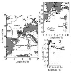
MM5 is run over 3 nested domains with respective horizontal resolutions of 27 km, 9 km and 3 km.
