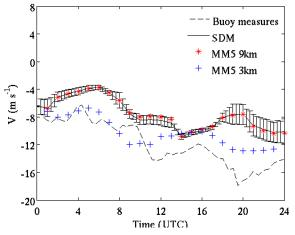
Comparison of MM5 at several scales, the buoy, and SDM in the cell containing the buoy.
