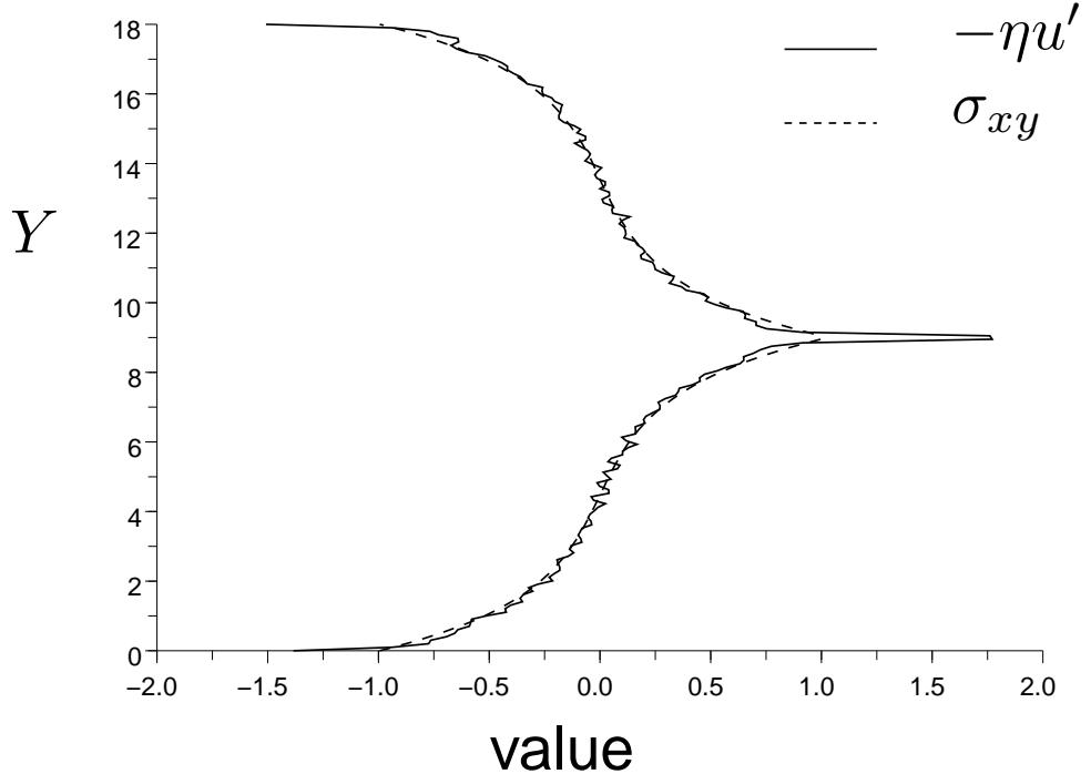
Velocity profile and off diagonal component of the stress tensor for the piecewise constant nongradient force.
