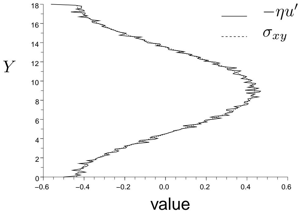
Velocity profile and off diagonal component of the stress tensor for the sinusoidal nongradient force.
