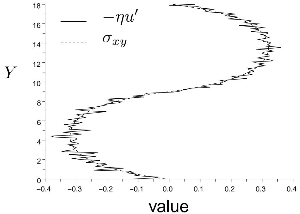
Velocity profile and off diagonal component of the stress tensor for the piecewise linear nongradient force.
