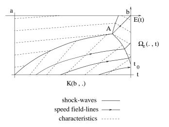
On this figure, the upstream demand has been assumed nil (this is the extreme possibility), hence the trajectory originating at (a, t) and the shockwave originating at the same point are coincident till point A. From point A on, traffic conditions imposed by the value of the downstream supply prevail along the trajectory originating at (a, t).
