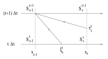
The field-line of  $\tilde{\mathcal{V}}$  originating at point  $(x_{s-1}, (t+1)\Delta t)$  of the space  $\times$  time  $(\xi, \tau)$  plane intersects either the line  $\xi = x_s$  at point  $(x_s, \tau_s^t)$ , or the line  $\tau = t\Delta t$  at point  $(\xi_s^t, t\Delta t)$ , depending on the relative value of  $V_s^t$ .
