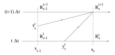
In the space  $\times$  time plane, which shall be denoted here the  $(\xi, \tau)$ -plane, the field-line of  $\mathcal{U}$  originating at point  $(x_s, (t+1)\hat{\Delta}t)$  intersects the line  $\xi = x_{s-1}$  at point  $(x_{s-1}, \tau_s^t)$ , or the line  $t = t\Delta t$  at point  $(y_s^t, t\Delta t)$ , depending on the relative value of  $V_s^t$ . Let us consider first intersection point  $(y_s^t, t\Delta t)$ . This point is given by
