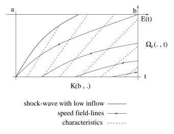
To construct the above figure, a low but non-zero demand has been used for illustrative purposes. If the demand were exactly nil, the shock-wave would be coincident with the trajectory originating at point (a, t).
