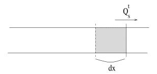
the outflow during a time step,  $Q_s^t \Delta t$ , will thus be equal to the mean cell density  $K_s^t$  times the distance covered during the time-step at speed  $V_s^t$ , i.e.  $K_s^t V_s^t \Delta t$ , which is the precise translation of the FIFO hypothesis if the density is assumed uniform in cell (s). Associated to this cell exit speed, it is possible to define the following ratio:
