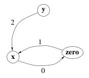
An important fact to notice about the weight of an edge is that its role is to represent the *maximum* weight between two nodes: suppose we have the two inequalities  $x \ge y + 1$  and  $x \ge y + 2$ , we will draw an edge of weight 2 from node x to node y, since the second inequality is more restrictive (and hence gives more information) than the first.
