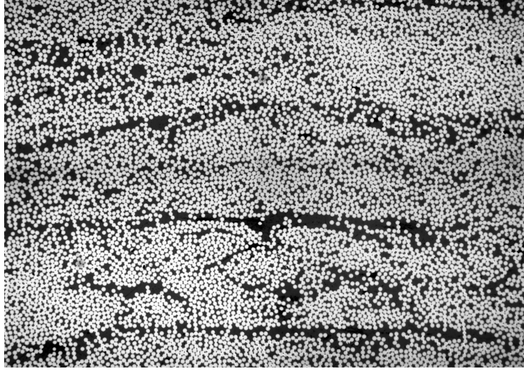
FIG. 2.2 – Two-dimensional cut of a composite material used in the aeronautics industry, extracted from [100] and reproduced with permission of the author. It is clear that this material is not periodic, yet there is some type of underlying periodic arrangement of the fibers.
