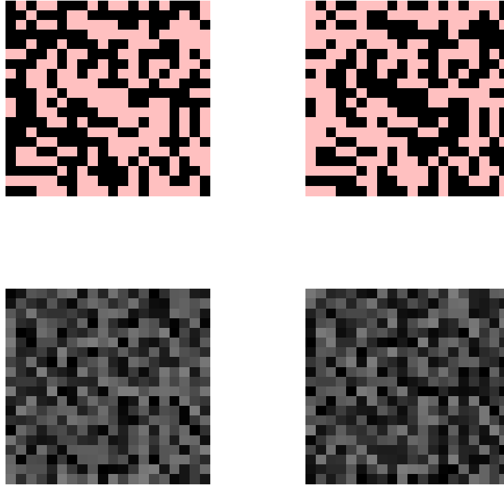
FIG. 3.1 – Realization of a(x, \omega) given by (3.2) (left) and the associated antithetic field b(x, \omega) (right). Top figures : a_0 \sim \mathcal{B}(1/2) ; bottom figures : a_0 \sim \mathcal{U}([\alpha, \beta]) .
