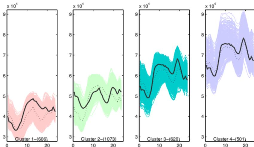
Figure :  $T = 2800$  intra day load curves of size  $n = 48$  (clustering using  $S = 7$  approximated coefficients)
