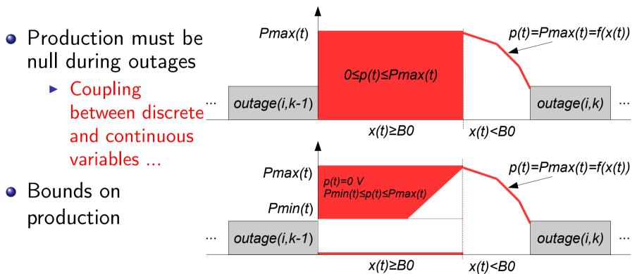
NB : after the "Zero Boron" threshold, non-linear decreasing profile depending on the stock  $\rightarrow$  Numerous state variables mandatory to impose the exact command...
