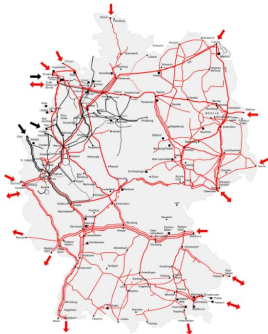
Figure: German H-gas and L-gas network system
