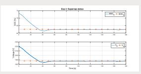
The SOC and voltage of the supercapacitor (blue line) with respect to their reference values (dotted red line).
