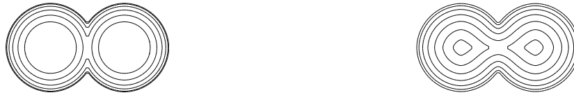
Fig. 5. Increasing (left) and decreasing (right) evolution of two circles by classical FD scheme
