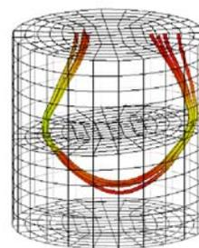
Figure 3 : Loops of currents in cryolite while metal pad rolling. We show here some streamlines of the field  $j$  (the perturbed current). The perturbed current goes from the right-hand side (where the elevation of the interface is the highest) to the left-hand side.
