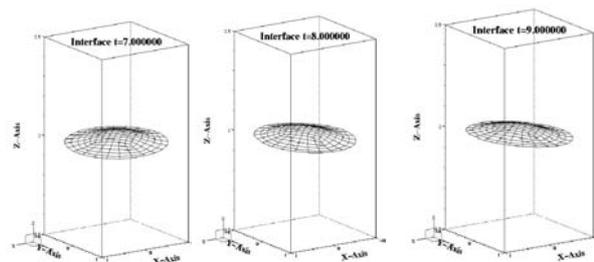
Figure 2 : The phenomenon of metal pad rolling in a circular cell. Visualization of the interface. This is a case with  $B_z > 0$  and no instabilities
