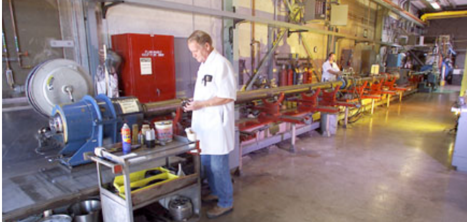
1) Two-stage gas gun (Livermore) 20 GPa in deuterium
