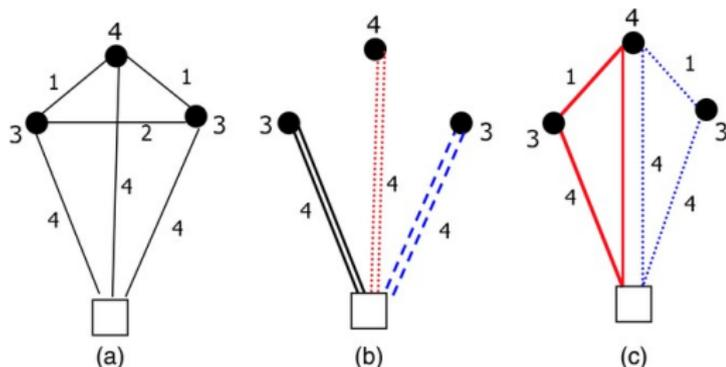
Instance (a) with  $Q = 5$ . The cost is 24 (with 3 vehicles) for the CVRP (b) and 18 (with 2 vehicles) for the SDVRP. Source: [Archetti and Speranza, 2012].
